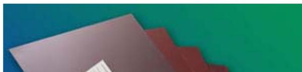
Key circuit materials to compare include relative permittivity or dielectric constant (also known by the abbreviation of  $\epsilon_r$ ), dissipation factor, thermal conductivity, glass transition
