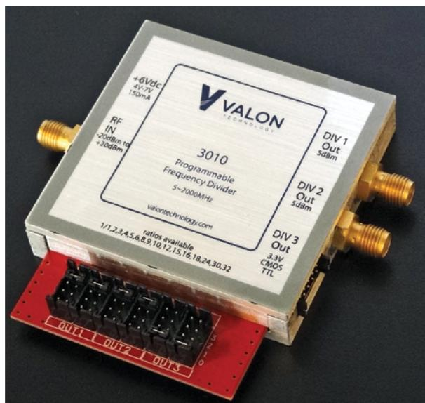
**2. Additional programmability and functionality in turn required a larger package for this analog/digital frequency divider.**
